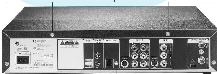
Figure 12-2: Remove only the screws holding TiVo's cover to its chassis, being careful not to remove any other screws.
